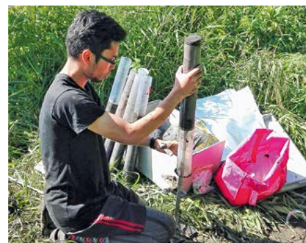
35 cm of sediment core samples were collected by using a sediment corer
